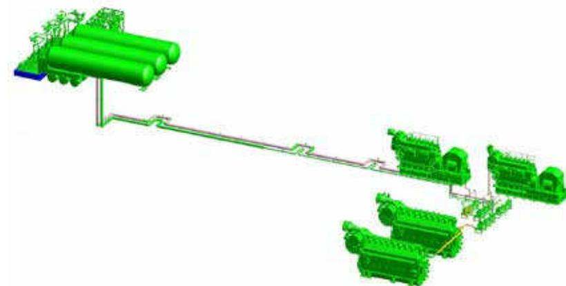
A model of the connection of LNG tanks and engine room...
